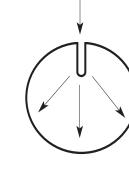
Protection may also be gained by pouring powdered PeneTreat into the kerf (0.2 to 0.3 pounds per lineal foot). Pour water into the kerf to dissolve and carry the PeneTreat into the wood. Brush or spray the exterior of the logs with more PeneTreat after either of these methods as described above.
